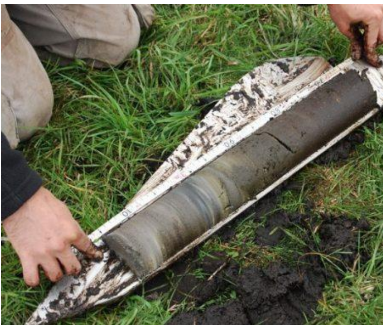
Fig 2: Collecting Soil Sample for Preliminary Soil Exploration
